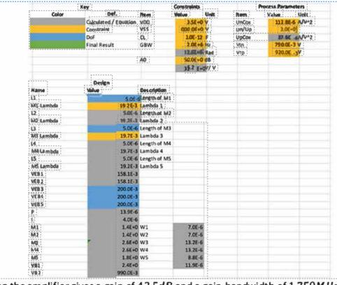
Simulating the amplifier gives a gain of 42.5dB and a gain-bandwidth of 1.759MHz. This is below spec but is improved by decreasing  $V_{EB1}$ ,  $\lambda_1$ , and  $\lambda_3$  further.
