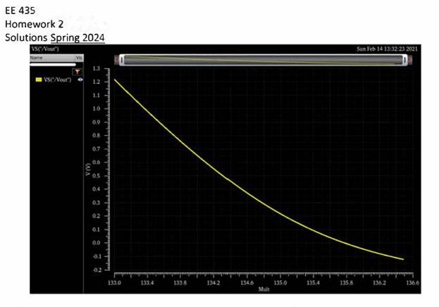
Adjusting our work slightly shows that a width-length ratio of 134.3 yields a quiescent output voltage of 507mV, which is well within 2.5% of the desired 0.5V point.
